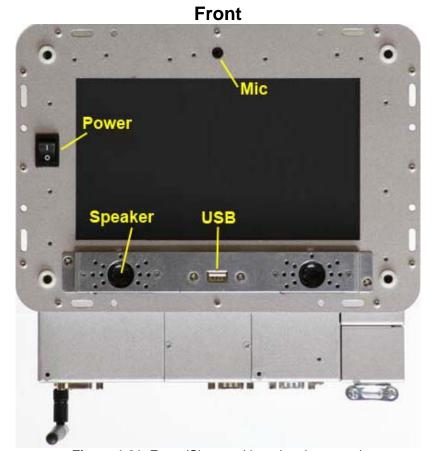
Figure 1.21 Front (Shown with optional antenna)
