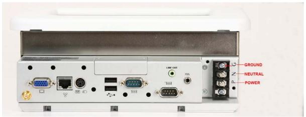
Figure 1.1 I/O Ports
